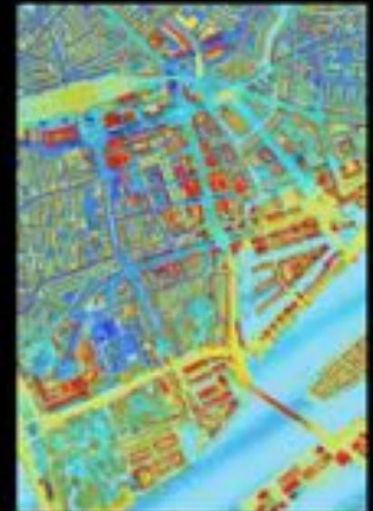
DLM of a section of Rotterdam. High definition elevation data obtained from airborne/laser scanning. Precision of about 20 cm per square meter, up to 20 measuring points per square meter
